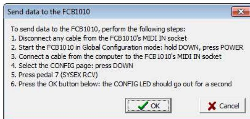
After you have pressed the OK button, the green CONFIG LED on the FCB1010's display should go out for about a second, then on again: this indicates that the FCB1010 has received the data. You must then press the DOWN pedal for about three seconds: this makes the FCB1010 actually *store* the received data, and terminate Global Configuration mode.
